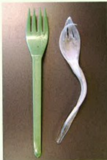
Synterra grade IM (left) and traditional PLA (right) after immersion in boiling water.
